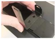
1. Turn the QuarterMaster upside down and attach the QuarterMaster / G2 brackets to the bottom of the unit with the screws provided. For the G2 the same applies. The long leg of the bracket goes to the front (blank) side of the QM, and the short leg goes towards the back (send & return) side.
