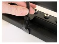
4. Secure the brackets with the re-usable cable ties that are provided as part of the kit. Trim any excess tie wrap.
