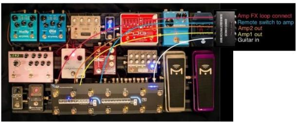
In the above example you can see how I'm using 4 mono connections to connect the Guitar input, Amp1, Amp2 and Amp's Remote Switch to G2. The 'Amp FX loop connect' is done using a TRS (stereo) cable
