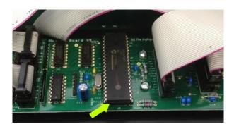
**Step 4** - Lever out the chip with a pair of tweezers.
