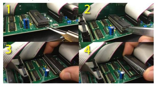
**Step 5** - Grab your new software chip. It's important that when you place the chip in the socket the small dimple needs to be closest to the back board.
