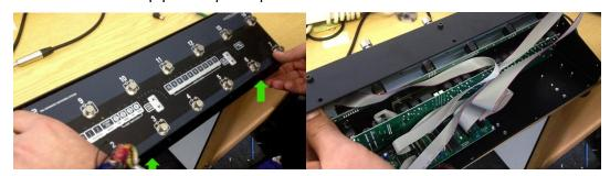
**Step 3** - Locate the software chip on the motherboard.
