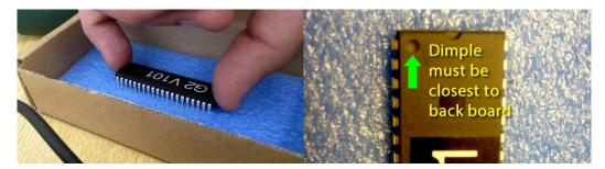
**Step 6** - Using the tweezers insert the software chip. Make sure all the pins are inserted. Apply even pressure and make sure the chip is fully inserted and all pins are socketed.
