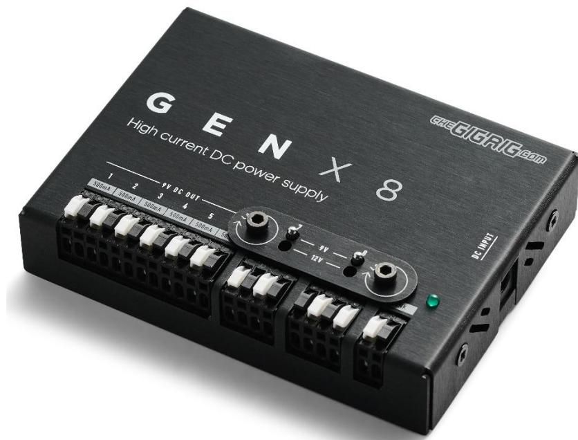
**LOCK GUARD:** To ensure you don't accidentally send the wrong voltage into any of your expensive pedals we've provided a **LOCK GUARD** on the switch. If you want to swap the voltage simply undo the two hex screws, remove the lock guard, and flick the switch. Reattach the **LOCK GUARD** once you've changed the voltage.
